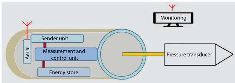
**Fig. 2:** Modular layout of the measurement system – main components
