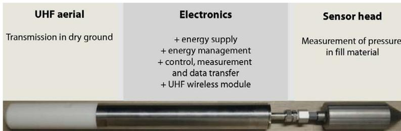
**Fig. 7:** General view of pressure transducer with wireless data transmission
