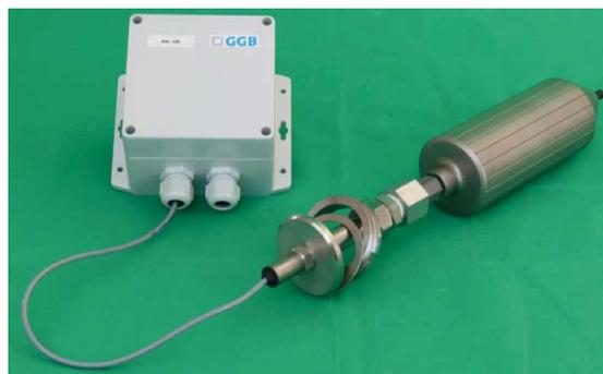
**Fig. 6:** Functional model components for wired in-situ tests
