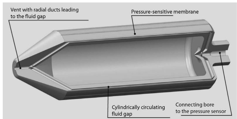
**Fig. 1:** Layout of the cylinder sensor head (CAD model)
