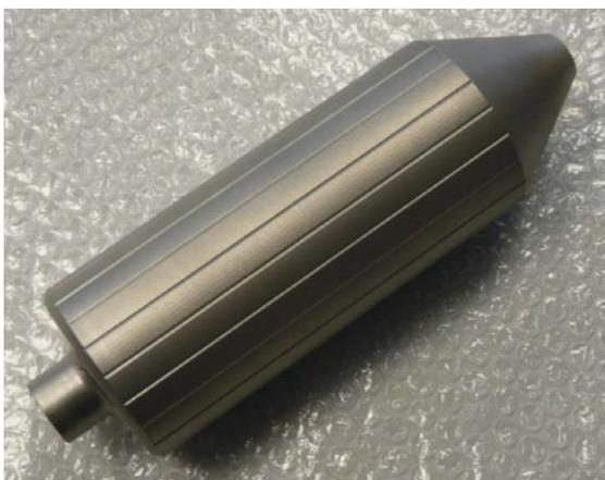
**Fig. 5:** View of sensor head after 3D printing
