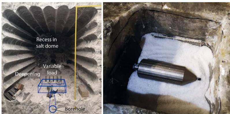
**Fig. 9:** Installation site of rock-pressure sensor for test arrangement 1
