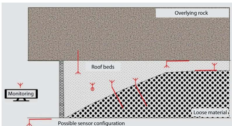
**Fig. 3:** Depiction showing different situations where the measurement system can be installed below ground
