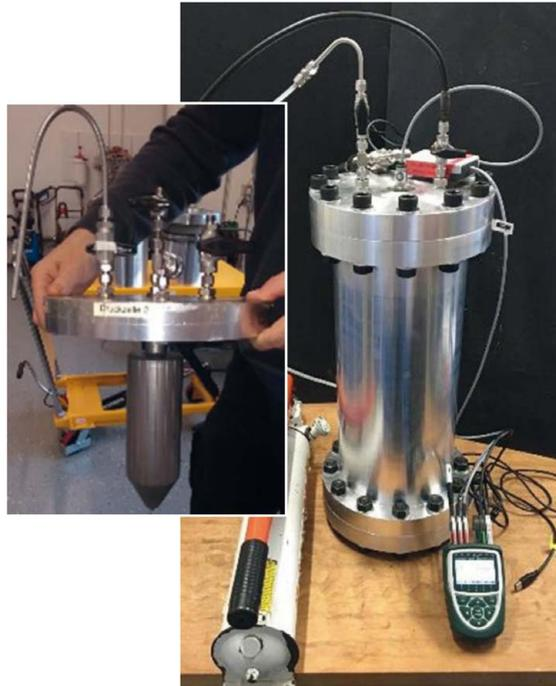
**Fig. 8:** Test set-up for calibration in the pressure autoclave
