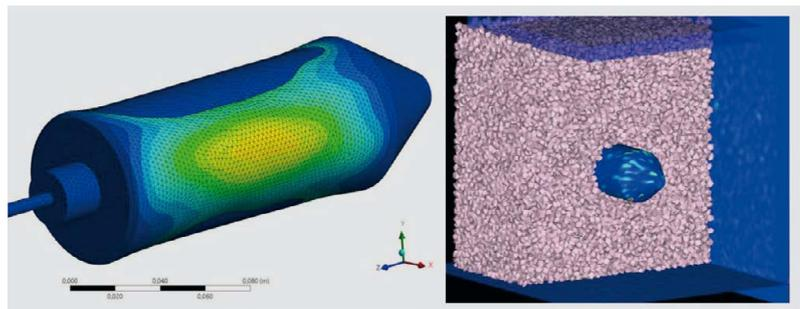
**Fig. 4:** Deformation of the cylinder barrel on taking on external load (pressure field) from the bedding material (depiction of deformation greatly exaggerated)
